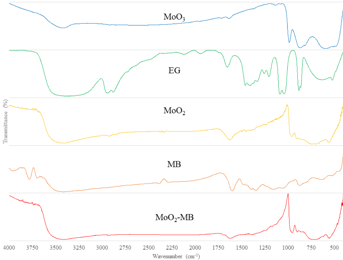
Figure 3.11 FTIR data showing the functionalization of MoO 2 .
